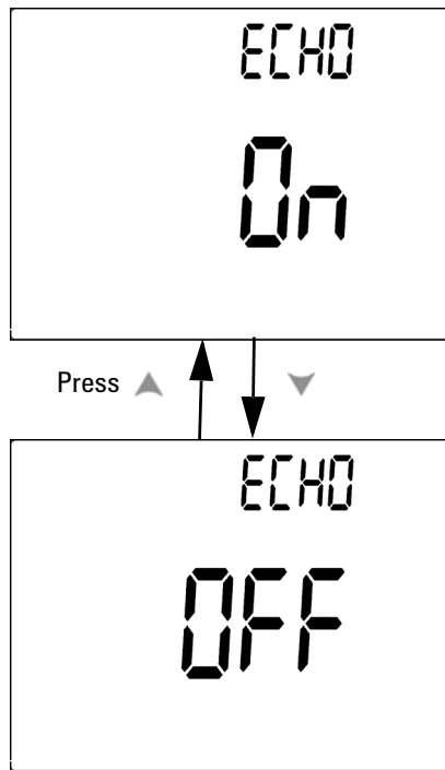
Figure 4-14 Echo mode setup for remote control
