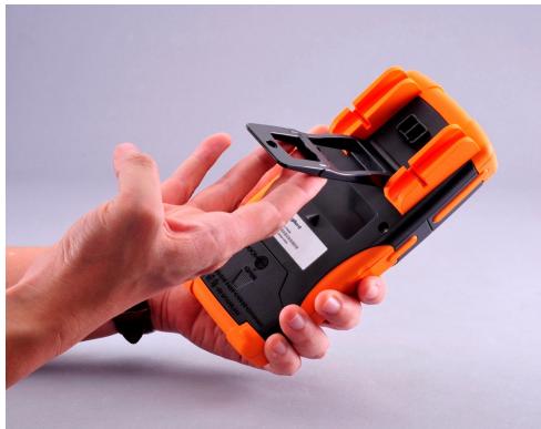
1. Extend the tilt-stand until its maximum reach
