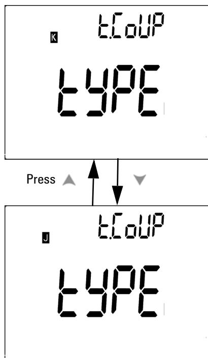
Figure 4-3 Thermocouple type setup
