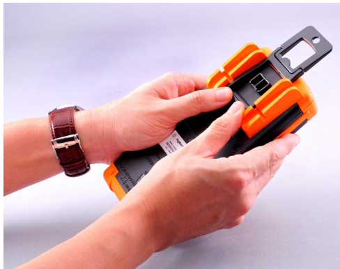
4. Re-attach the tilt-stand to an upright position
